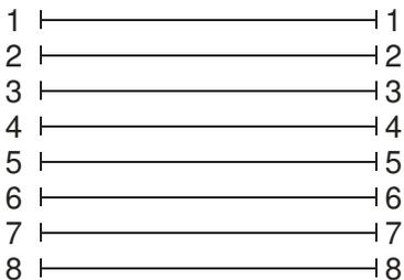
The speed of the data transmission between the XRC-CT15b and the XRC-150/200 is 250 kBaud. Therefore, the cable mustn't be very high quality.
