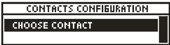
Now you need to choose the contact by activating it. For example if you have connected a switch on contact1, press this switch to configure contact1:
